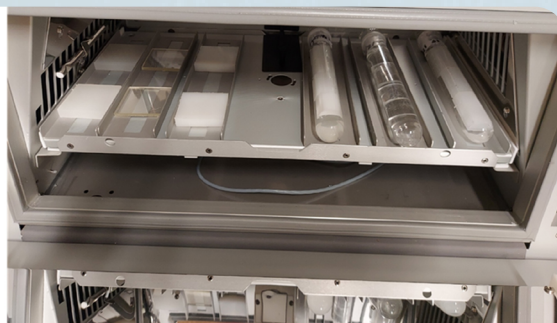
The different materials will be artificially aged using a Q-SUN Xenon test chamber.
