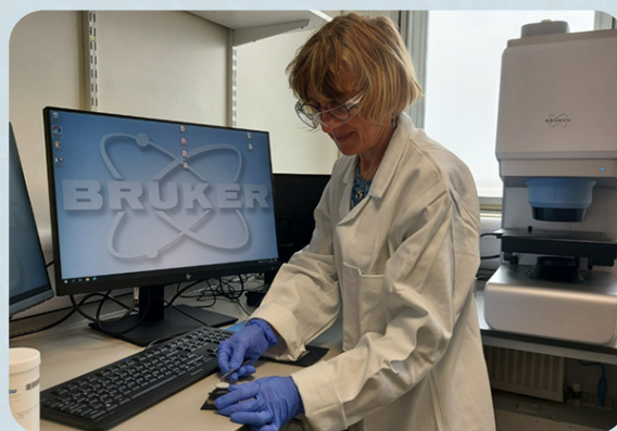
Microplastic analysis using a Bruker LUMOS II micro-FTIR.
