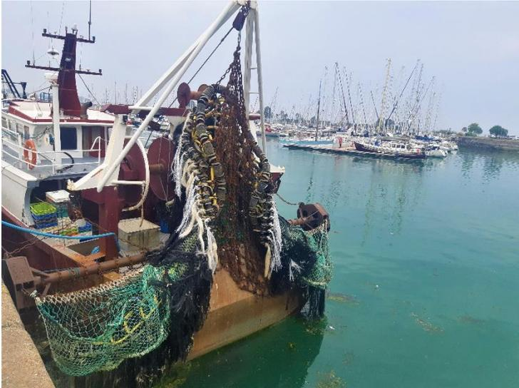
Figure 32 – Beam trawl ready for fishing
