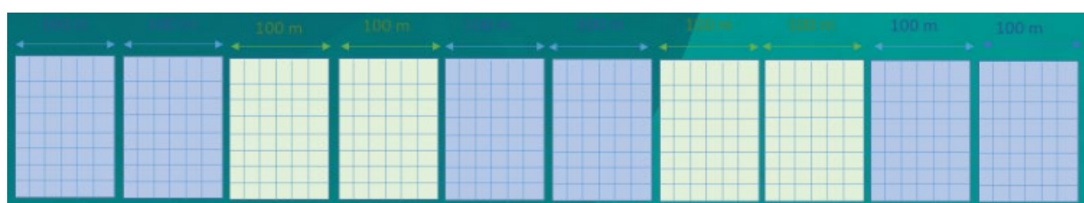
Figure 17: Proposal 1: Alternate INdIGO and nylon nets every 200 meters
