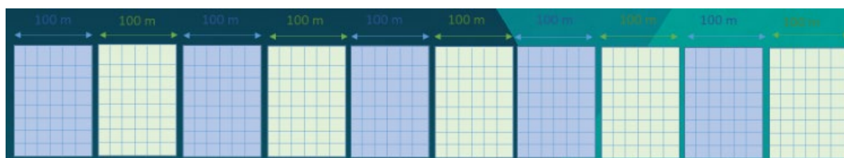
Figure 18 : Proposal 2: Alternate INdIGO and nylon nets every 100 meters
