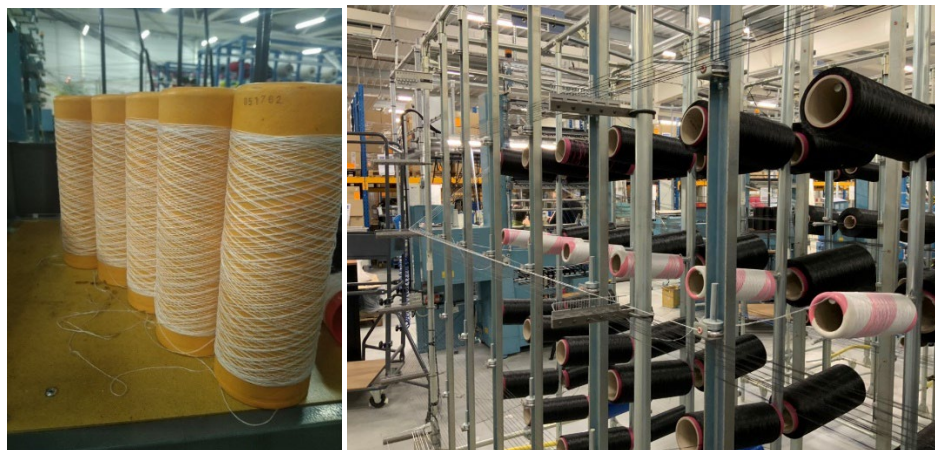
Figure 3 : Illustration of stages 1 and 2, with the coils being cut (left) and loaded onto the machine (right).
