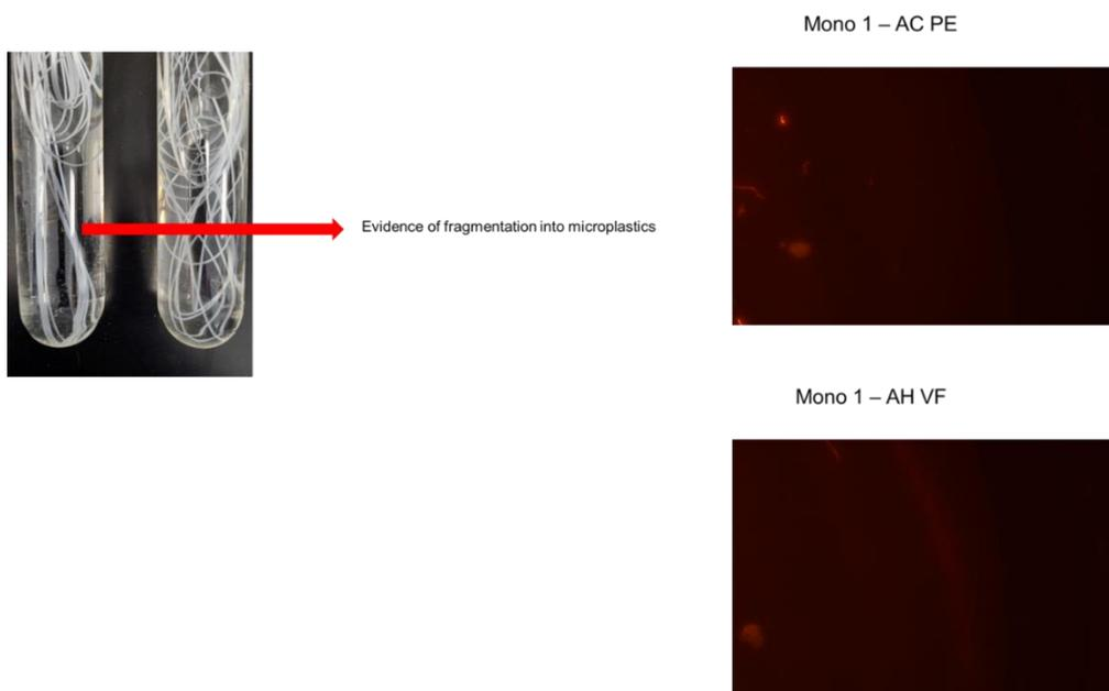
Figure 28. Evidence of fragmentation of the monofilaments as confirmed by micro-FTIR.
