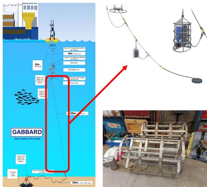
Figure 4: Deployment configuration at sea for ageing INdIGO samples.
