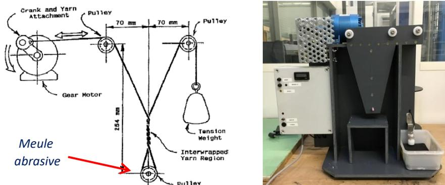
Figure 11: Diagram corresponding to the ASTM standard where abrasion takes place filament against filament (left) and machine used with an abrasive surface instead of a pulley (right)
