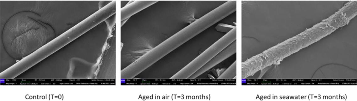
Figure 22 : Microscopic observations of the surface condition of monofilaments and multifilaments before and after accelerated ageing exposed to air and seawater in the ageing chamber (magnification x100).
