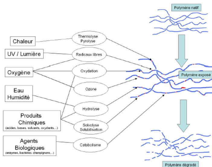
Figure 10: Major polymer degradation agents leading to changes in molecular mass.
