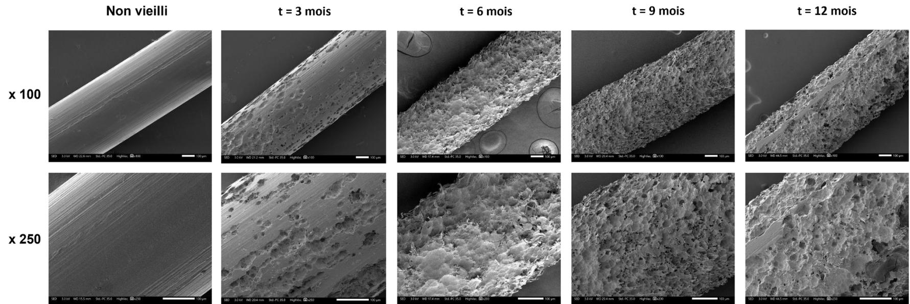
Figure 13: Microscopic observations of the surface condition of AH monofilaments before and after natural ageing in a marine environment at two magnifications (x100 et x250)
