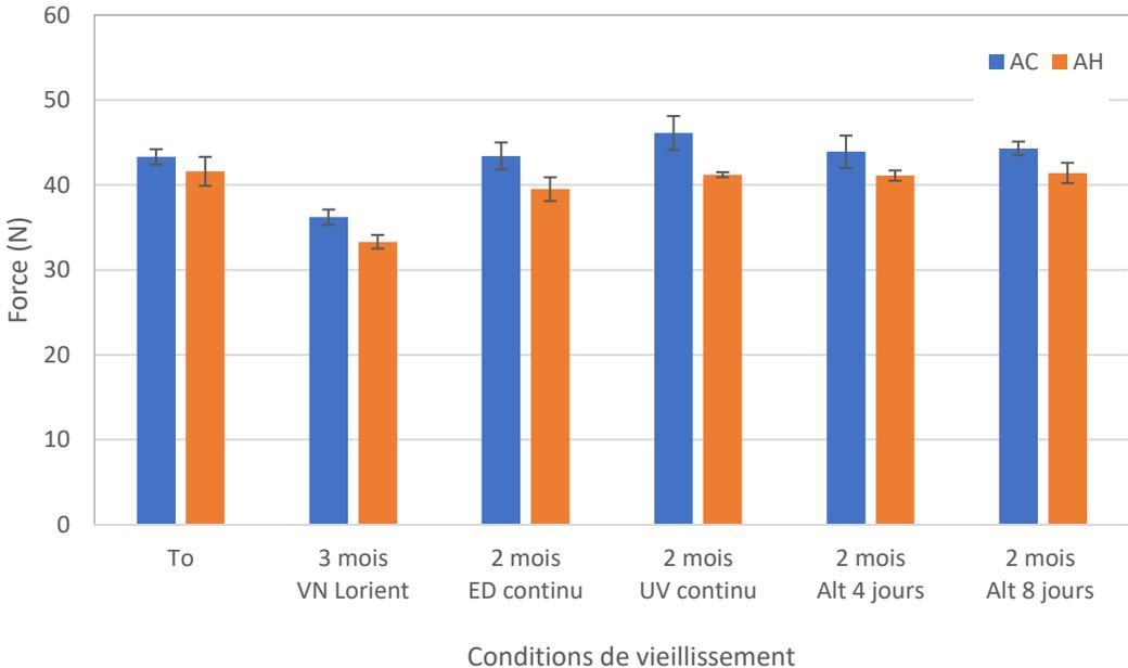
Figure 24 : Comparison of the evolution of the breaking strength of AC and AH monofilaments as a function of the ageing conditions studied over short periods of time.
