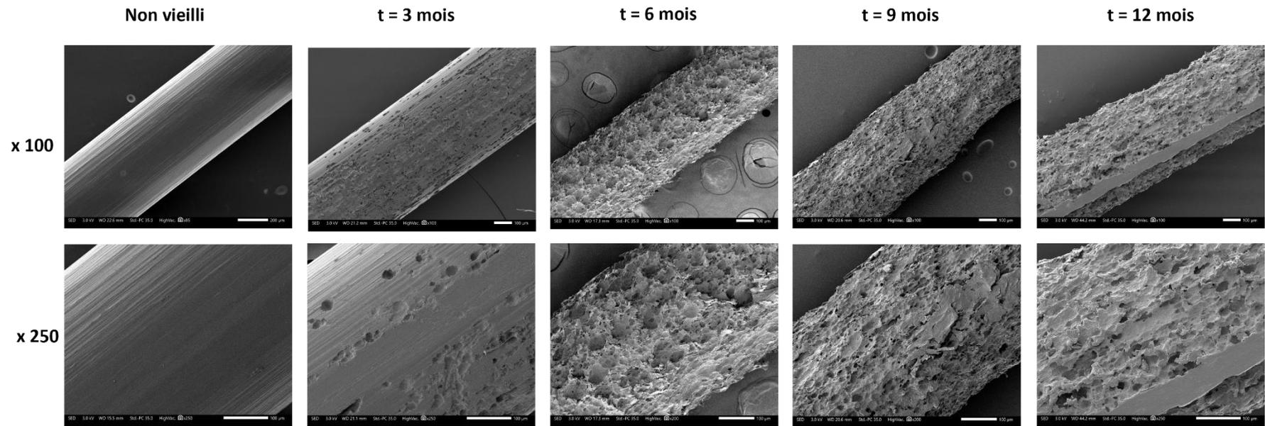
Figure 12: Microscopic observations of the surface condition of AC monofilaments before and after natural ageing in a marine environment at two magnifications (x100 et x250)
