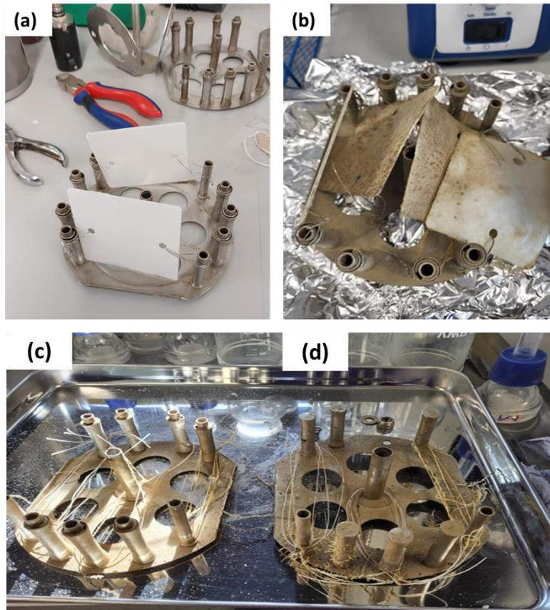
Figure 18. Fixation of samples before deployment (a/ b) and after deployment at sea (b/ d) for samples in the form of plates (a/ b) and mono and multifilaments (c/d).
