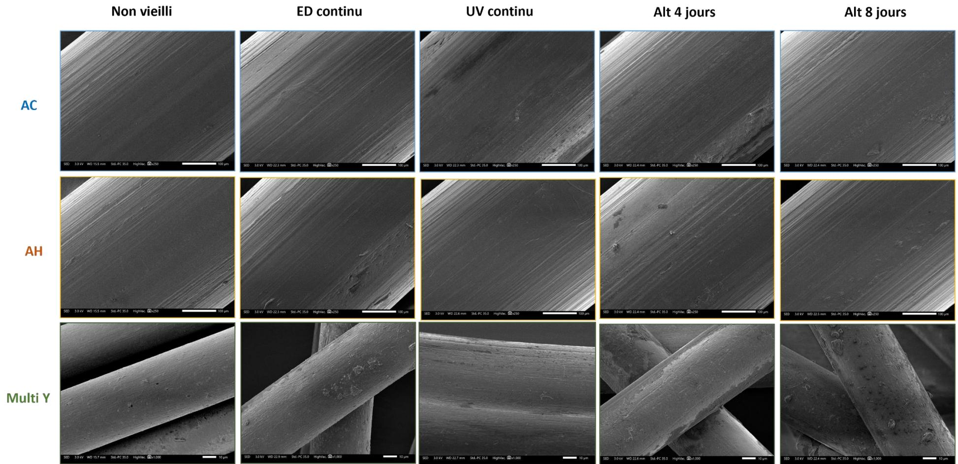
Figure 23 : Microscopic observations of the surface condition of AC and AH monofilaments (magnification x250) and Y multifilaments (magnification x1000) before and after continuous ageing (ED = distilled water and UV) and alternating ageing (Alt 4 and 8 days).
