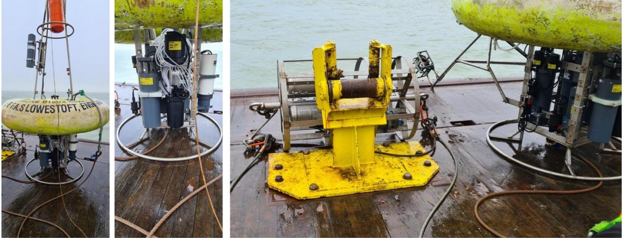
**Figure A2.** Deployment of the mid-tether frame alongside the SmartBuoy.
