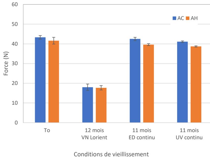
*Figure 25 : Comparison of the evolution of the breaking strength of AC and AH monofilaments as a function of the ageing conditions studied over extended periods of time.*
