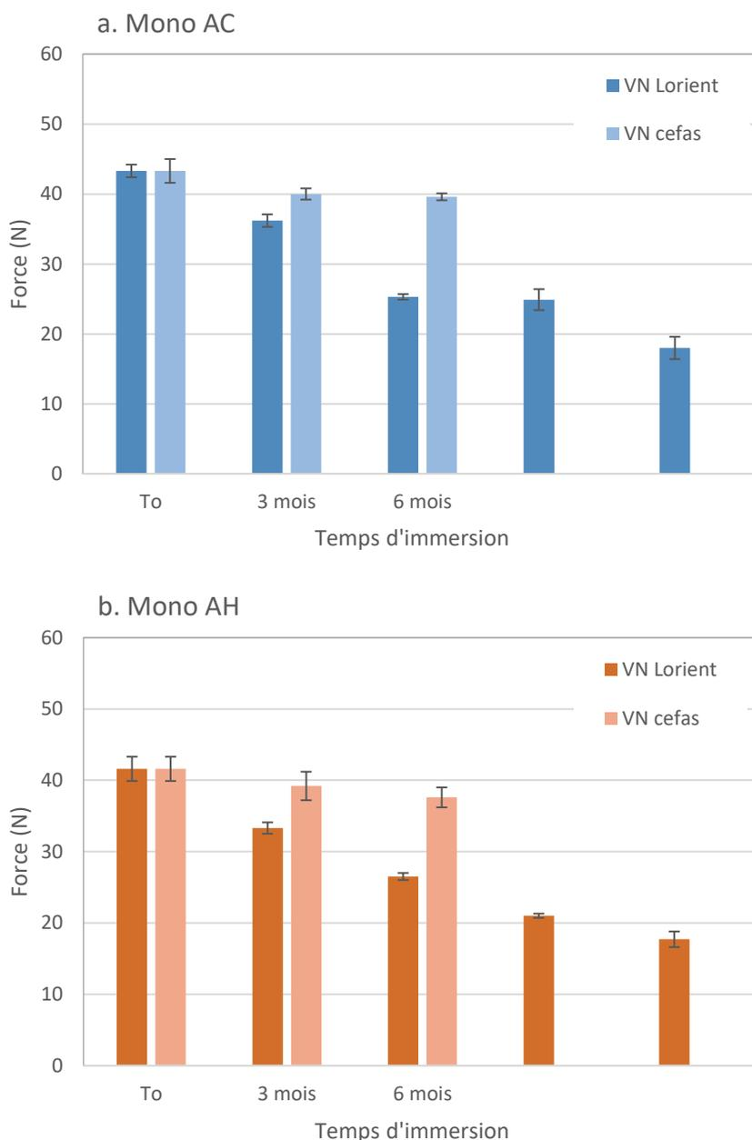
Figure 19: Comparison of the evolution of the breaking strength of AC (a) and AH (b) monofilaments as a function of the immersion environment: natural ageing at Lorient and natural ageing at Cefas.
