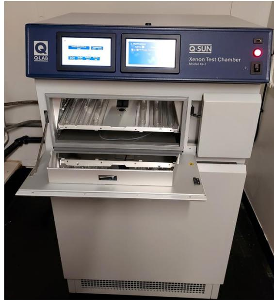
*Figure 9: Q-SUN ageing chamber for accelerated ageing of biodegradable materials.*
