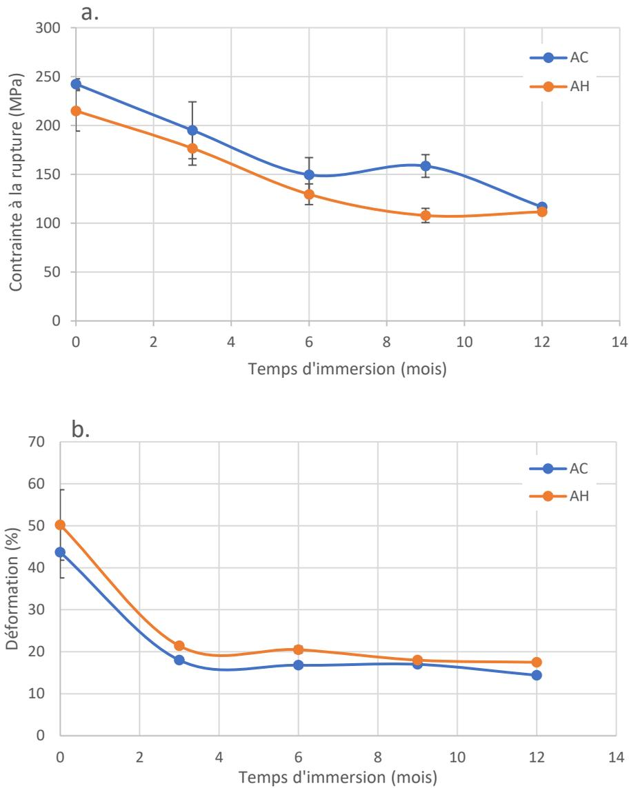
Figure 16 : Evolution of stress at break (a) and strain at break (b) as a function of immersion time in natural seawater for AC and AH monofilaments.
