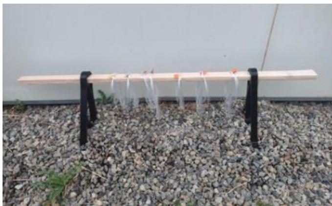
Figure 7: Mounting for exposure of wires to the sun's UV rays with natural ageing.
