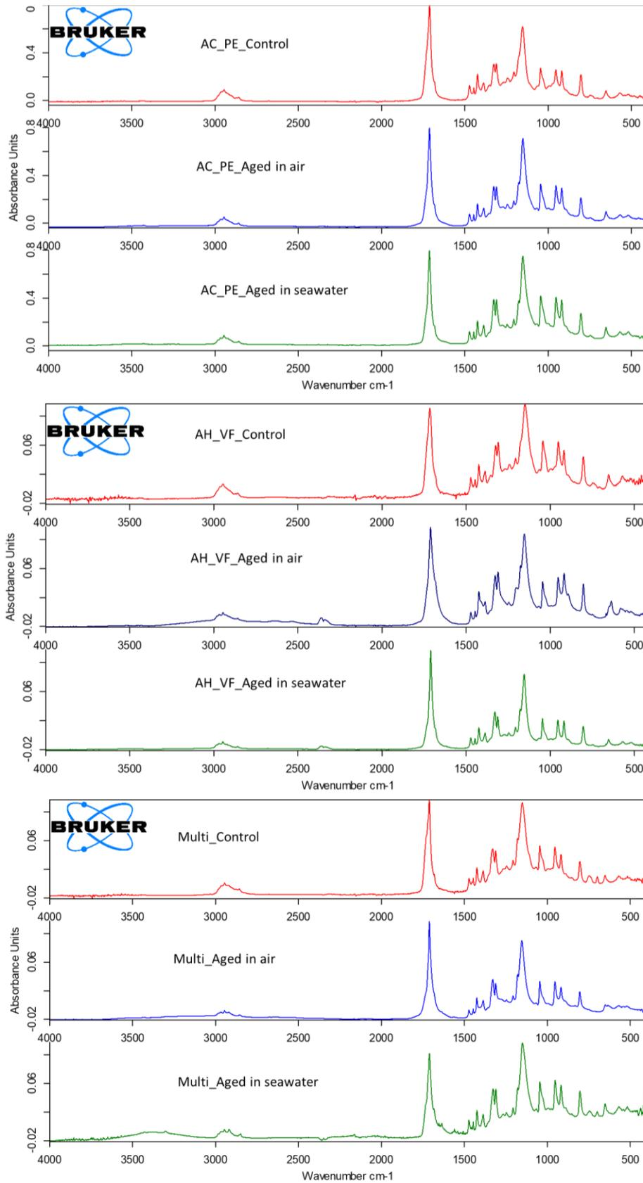
Figure 21. ATR-FTIR profiles of the mono and multi-filaments after ageing in air for 3 months using the Xenon-test chamber.
