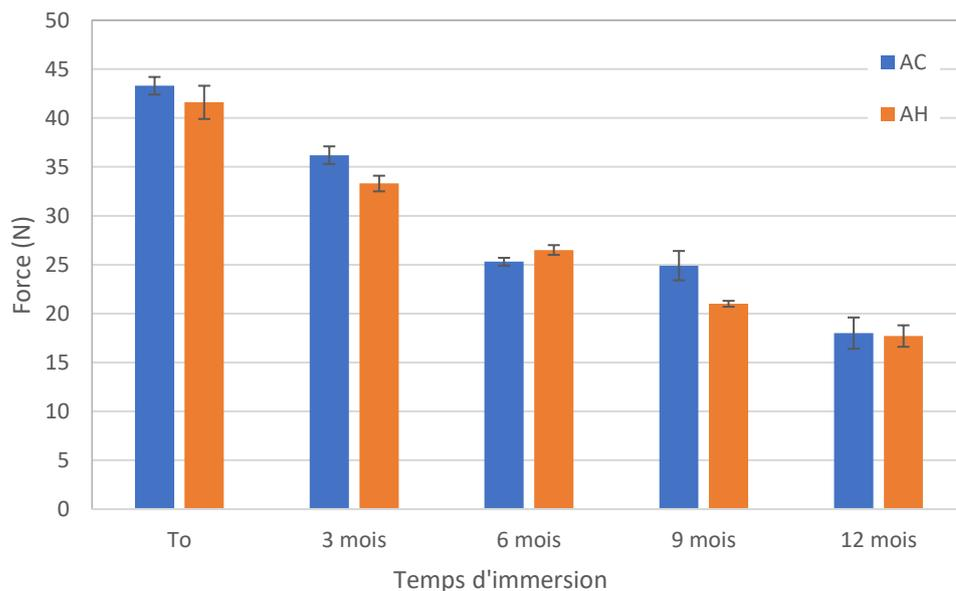
Figure 15 : Progressive changes in the breaking strength of the 2 monofilaments studied
