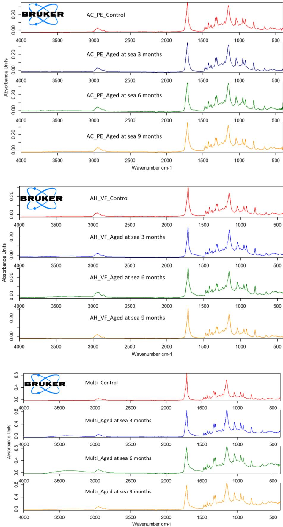
Figure 20: Infrared spectra of AC, AH monofilaments and biodegradable multifilaments obtained before and after ageing as a function of immersion time.
