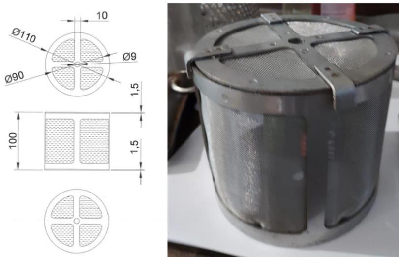
Figure 6: Sample cage for studying the fragmentation of microplastic materials.
