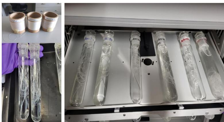
Figure 8: Exposure of materials in glass tubes installed in the ageing chamber.
