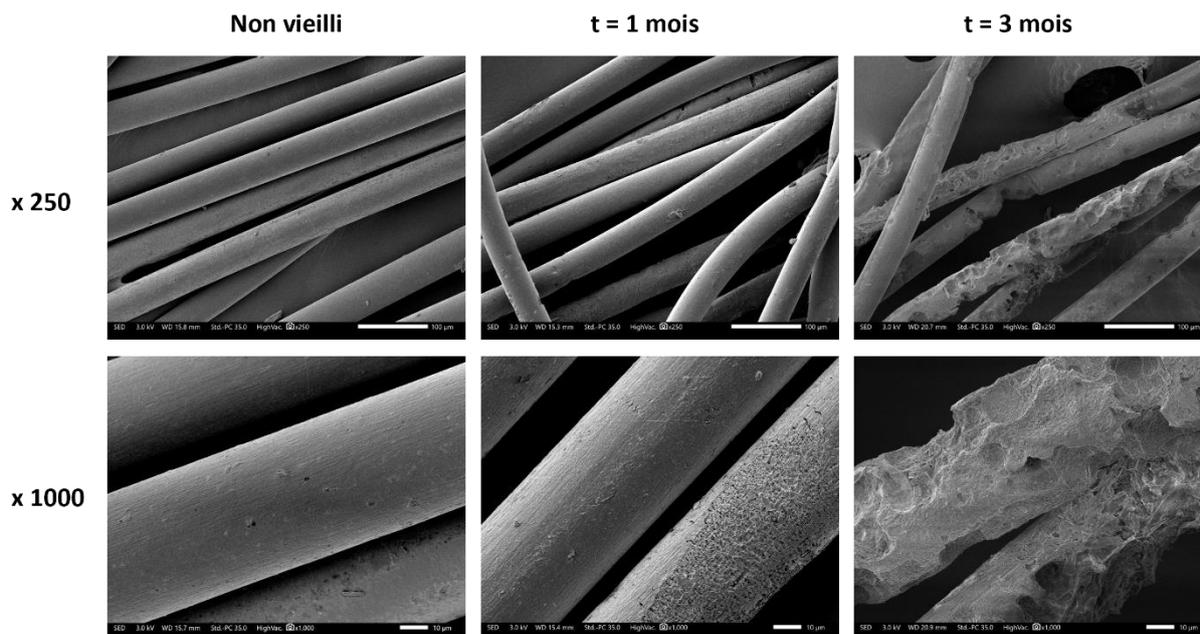
Figure 14: Microscopic observations of multifilaments before and after ageing in a marine environment.
