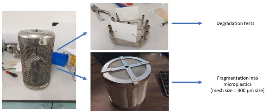
Figure 5: Modified passive sampling cage for the deployment of biodegradable materials at sea.
