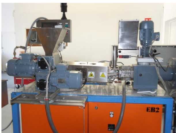
Figure 2: Twin-screw co-rotative extruder
