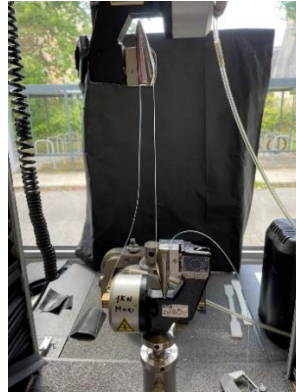
Figure 13 : monofilament installed on the traction machine before testing
