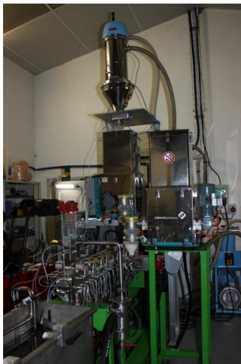
Figure 3: Twin-screw co-rotative extruder TSA FSCM 27-50
