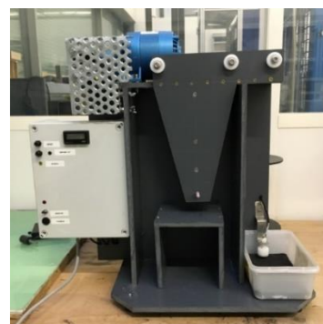
Figure 14: Diagram corresponding to the ASTM standard where abrasion takes place filament against filament (left) and machine used with an abrasive surface instead of a pulley (right)
