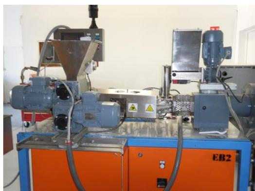
Figure 2 : Extrudeuse bi-vis co-rotative
