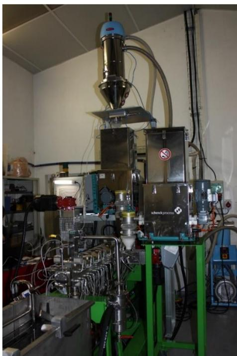
Figure 3 : Extrudeuse bi-vis co-rotative TSA FSCM 27-50
